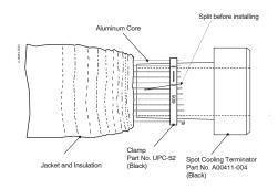
Note — When connecting the supply tubing to the outlet, it is necessary to slit the tube end so it fits over the stub. Then use the clamp and seal the connection as you would for all outlets.
