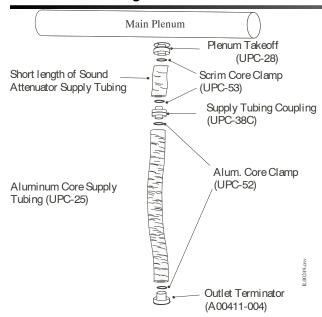
The plenum should be made of metal (minimum 26 ga) as it is sturdier and the takeoffs are much more secure. It is important, though, to seal the metal duct and to insulate the duct with at least 1.5 inches of blanket fiberglass or insulation sleeve. Also, be sure to use a foam saddle under the duct wherever it is supported by a strap. The plenum should be designed the same as the current Unico System layout (Bulletin 30-01).
