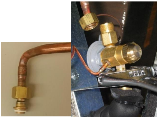
Figure 25. Install White Teflon O-ring in both connections (not on iSeries). Attach and tighten lower connecting nut
