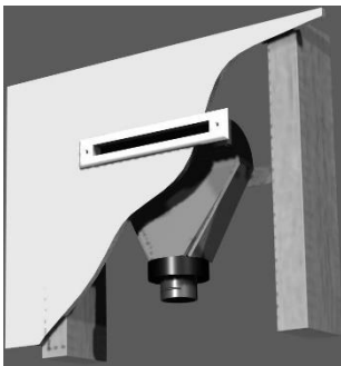
Figure 3. Typical Wall Installation, 90° Outlet
