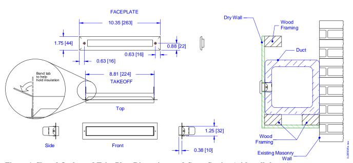
Figure 1. Slotted Outlet and Trim Plate Dimensions and Cross-Section (with wall shown)
