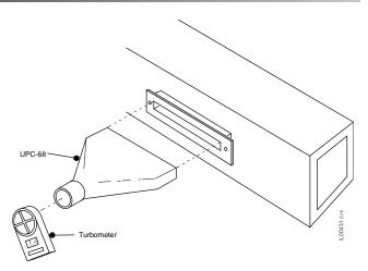
Figure 3. Measuring airflow.
